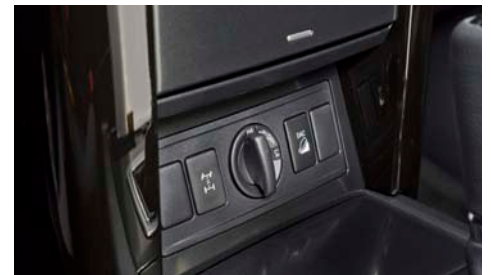
All models feature Downhill Assist Control (DAC) to keep descents under control. There's also a centre diff lock switch that ensures all wheels work together.
