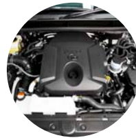
2.8 Litre Turbo Diesel 4 cylinder DOHC and Common Rail Direct Injection (D-4D)
