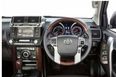
The 4 spoke leather steering wheel features premium quality wood-grain detailing and houses controls for the audio system, Multi-Information Display (MID), Dynamic Radar Cruise Control (DRCC), and Bluetooth voice controls.
