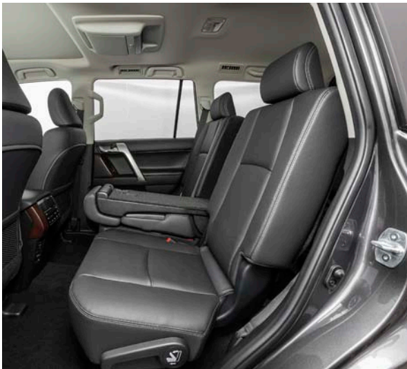
The tri-folding 2nd row seats feature a simple lever-operated walk in entry system to allow passengers quick access to 3rd row seating.
