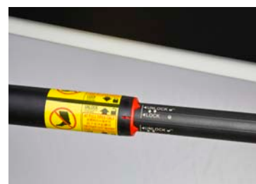
Toyota's attention to detail extends to the conveniently located wheel changing kit, stored within a panel in the rear cargo door. The rear door won't close on you, even if you're parked on an unfavourable grade, thanks to this lockable strut, keeping the door open so you can load up easily. A top hinged glass tailgate hatch gives access to the vehicle's load space even in tight spaces where full tailgate opening may be restricted.
