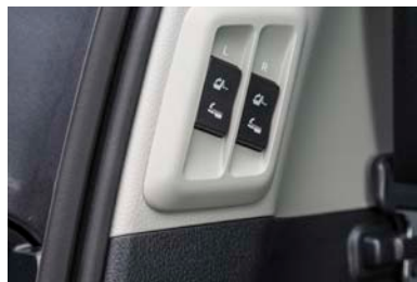
The 3rd row of seats can be raised or stowed flat automatically via buttons located within VX and VX Limited's cargo area. The 3rd row of seats are split-folding for added flexibility.
