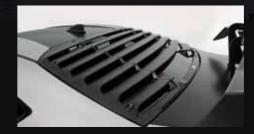
TRD Rear Window Louvre. Produces a powerful rear styling without greatly hindering the field of vision, as well as suppressing the penetration of sunlight into the room from above.
