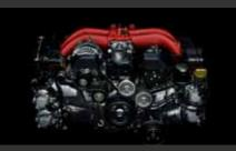
The boxer engine's naturally balanced four horizontally opposed pistons and square, 86mm x 86mm bore and stroke lie at the heart of the 86's design. The engine's low positioning allowed for the vehicle's ultra-low centre of gravity, and low-inertia cornering.
