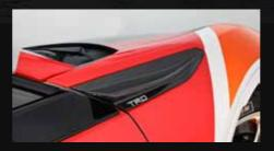
TRD Front Fender Aero Fin (CFRP). During driving the front fender fins improve the ground feeling by generating downforce at the front and give an improved stability feeling while cornering. The carbon fibre gives an increased strength to the fin while giving an attractive aesthetic to the side of the car.
