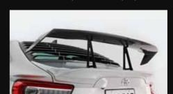
TRD GT Wing. This newly designed GT wing incorporates a swan neck mount allowing for a nice, smooth lower surface of the wing. This gives the driver excellent down force and therefore traction.
