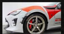
18" TRD 'SF3' (Forged) aluminium wheel. Newly designed Forged alloy wheel to which its 5 spoke design offers rigidity and has suitable weight reduction at only 8.2kg per wheel.
