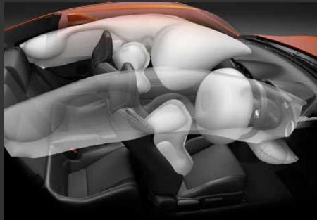
Seven airbags provide a comprehensive curtain of protection, including a driver's knee airbag.
