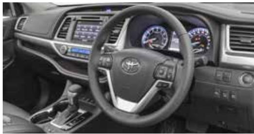
Steering wheel – leather with multi-information display, audio and phone controls with voice recognition, 4.2-inch colour multi-information display and illuminated combination meters
