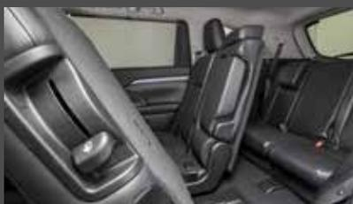
*60:40 split folding rear seating and four-way front passenger and second row manual adjustment*
