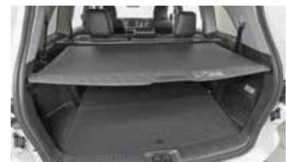
Cargo area – up to 1,872-litre capacity (behind first row). Four cargo hooks, carpeted deck board, moulded resin trim and extendable tonneau cover (shown)
