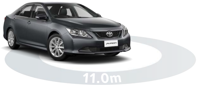
Electric Power Steering (EPS) is vehicle speed sensitive so low speed manoeuvres require minimal effort while at highway speeds less assistance is provided. The turning circle for Aurion AT-X is 11.0m and 11.4m for Sportivo ZR6.
