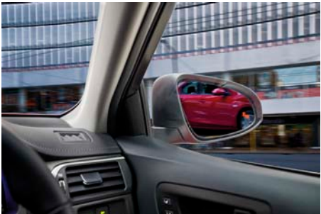
Aurion ZR6 safety features include a Blind Spot Monitor (BSM) that alerts the driver to vehicles in adjacent lanes, indicating their presence with lighted symbols in each exterior mirror. Additionally Rear Cross Traffic Alert (RCTA) uses radar when reversing to detect cross-traffic that may intersect your vehicle's pathway. RCTA sounds a warning and also flashes the outer lighted symbols.
