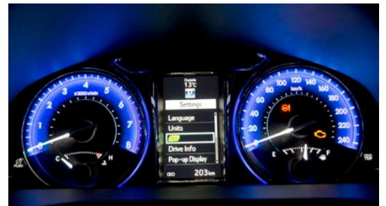
A dual dial speedometer with a 4.2" Multi-Information Display featuring range, average fuel economy, average speed, driving time and ECO Drive Level displays.
