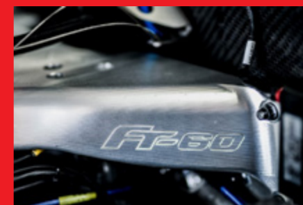
FIA Homologated Toyota 8AR-FTS, two litre, turbocharged, direct injection, 285hp (212 kW) engine.
