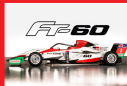
The FT-60 chassis is supplied by Tatuus in Italy and constructed to FIA Regional Formula 3 safety standards.
