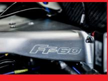
Toyota 8AR-FTS, two litre, turbocharged, direct injection, 285hp (212 kW) engine.
