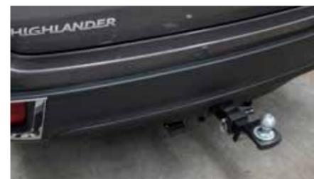
**Towbar and wiring harness.** This removable tongue tow bar and accessories allow you to tow a maximum braked load of 2000kg and unbraked load of 700kg. Tested to stringent standards you'll have peace of mind no matter what you tow.
