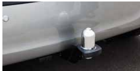
Towbar and wiring harness. Fixed tongue towbar rated to 900kg braked. Trailer wiring harness, towball and towball cover available - sold separately.
