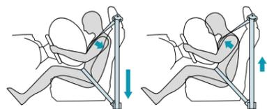
Front and outer rear seats have pretensioners and force limiters. Pretensioners instantly tighten the seat belts at the time of a collision to help enhance occupant restraint performance. The force limiter function loosens the seat belts while maintaining the load to help mitigate the impact to the chest regions of the front seat occupants.
