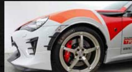
18" TRD 'SF3' (Forged) aluminium wheel. Newly designed Forged alloy wheel to which its 5 spoke design offers rigidity and has suitable weight reduction at only 8.2kg per wheel.
