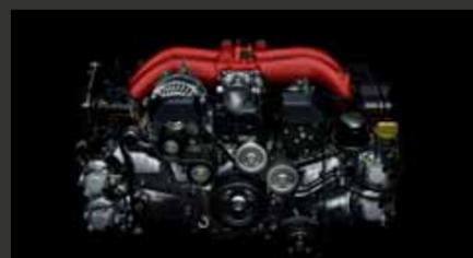
The boxer engine's naturally balanced four horizontally opposed pistons and square, 86mm x 86mm bore and stroke lie at the heart of the 86's design. The engine's low positioning allowed for the vehicle's ultra-low centre of gravity, and low-inertia cornering.
