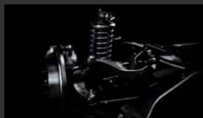
MacPherson strut front and lightweight but strong double wishbone rear suspension add extra grip and agility to an already perfectly balanced vehicle.
