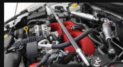
TRD Front tower bar. This tower bar features a carbon shaft for simultaneous optimal rigidity and weight reduction. It brings out the suspension's full performance by controlling flex in the upper part of the suspension tower. Even customers who choose not to replace their suspension will feel the boost in body rigidity. Install together with the member brace set and door stabilisers to take that body rigidity even further.
