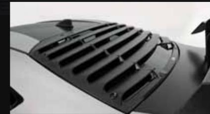
TRD Rear Window Louvre. Produces a powerful rear styling without greatly hindering the field of vision, as well as suppressing the penetration of sunlight into the room from above.
