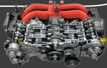
The 86's 2.0L front boxer engine has D-4S direct injection to provide you with power when you need it. With manual models the engine achieves a 152kW @ 7,000 rpm and 212Nm of torque @ 6400-6800 rpm. At 5000 revs the car's attitude changes and it's on!
