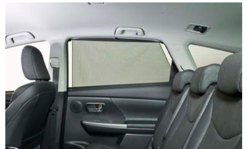
The rear side door and rear glass has privacy tinting. For extra privacy and protection the rear side doors have pull-up sunshades that help keep rear passengers cool in the summer months.
