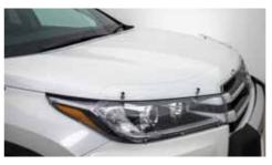
**Bonnet Protector.** This acrylic bonnet protector is custom-shaped to protect the bonnet from stone chips, insects and paint damage. Resistant to UV discolouration.
