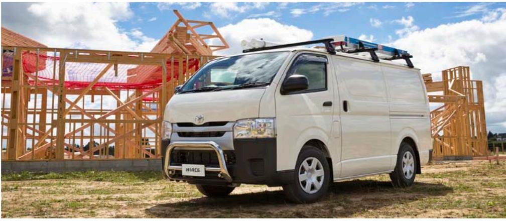
Hiace ZL full panel van shown fitted with nudge bar, weathershields, headlight protectors, rear bull bar, towbar and roofrack.
