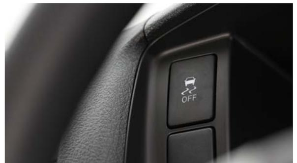
VSC (Vehicle Stability Control) helps you correct a loss of control by detecting if the vehicle is starting to skid or slide. By comparing the vehicle's direction of travel with your steering, acceleration and braking inputs it can tell if you are deviating from the intended direction. VSC then warns you, reduces engine power and controls the brakes to help you correct the situation.
