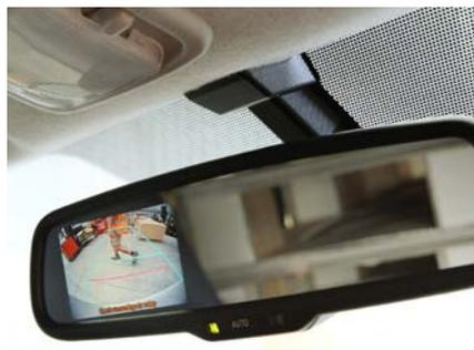
Each Hiace features a reversing camera with static guide lines and a clever colour monitor camera embedded in the rear view mirror, offering extra convenience in confined urban delivery zones and added peace of mind when reversing in residential areas.
