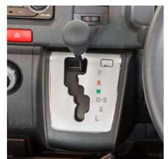
An important feature is the dash mounted gear lever that maximises interior space.
