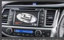
Eight-inch audio display with satellite navigation and monitor for reversing camera
