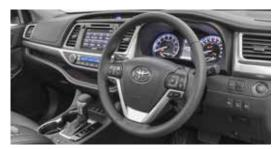
Steering wheel – leather with multi-information display, audio and phone controls with voice recognition, 4.2-inch colour multi-information display and illuminated combination meters
