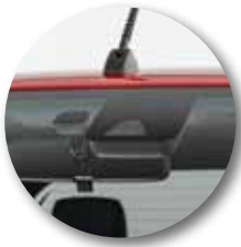
Toyota Safety Sense information is gathered by a forward facing camera and radar that analyse a wide range of data that aids in delivering added safety to Hilux.
