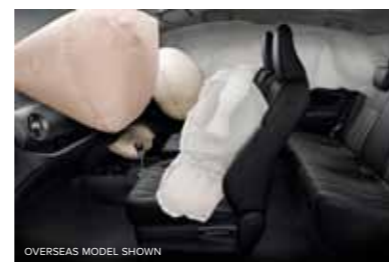
Yaris occupants are well protected with driver and front passenger, front seat side, front and rear curtain shield and driver's knee airbags.
