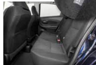
The rear seats have two ISOFIX fixing points enabling child seating to be easily attached. There are also 3 tether anchors.
