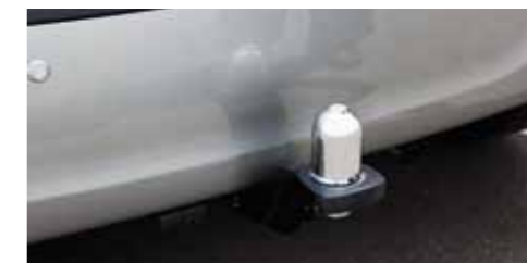
Towbar and wiring harness. Fixed tongue towbar rated to 900kg braked. Trailer wiring harness, towball and towball cover available - sold separately.
