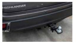
Towbar and wiring harness. This removable tongue tow bar and accessories allow you to tow a maximum braked load of 2000kg and unbraked load of 700kg. Tested to stringent standards you'll have peace of mind no matter what you tow.
