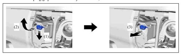
5. Carry the removed service plug grip in your pocket to prevent other staff from accidentally reinstalling it while you are dismantling the vehicle.
