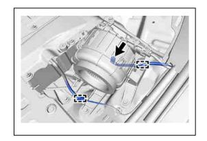
(3) Remove the 3 bolts to remove the battery cooling blower assembly.
