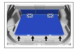
Remove the No. 4 HV battery shield panel.
