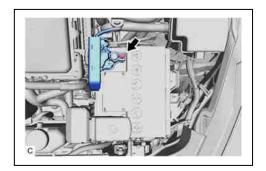
1. Disengage the 2 claws and open the battery terminal.
