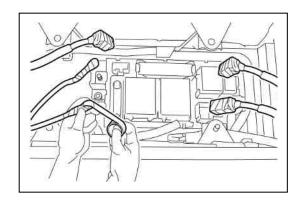
Check the HV battery and nearby area for leakage. If you find any liquid, it may be strong alkaline electrolyte. Wear rubber gloves and goggles and neutralize the liquid using a saturated boric acid solution or vinegar. Then wipe up the liquid using waste rags etc.
