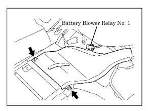
16 Remove battery bracket reinforcement.
