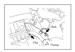
18 Remove battery carrier panel No. 6.
