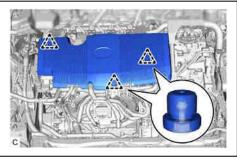
holding the left and right sides may cause the No. 1 engine cover sub-assembly to break.
