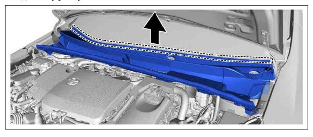
(3) Disengage the 4 guides and remove the cowl top ventilator louver sub-assembly as shown in the illustration.
