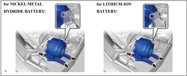
(4) Disengage the 2 claws to remove the battery cooling blower assembly.
