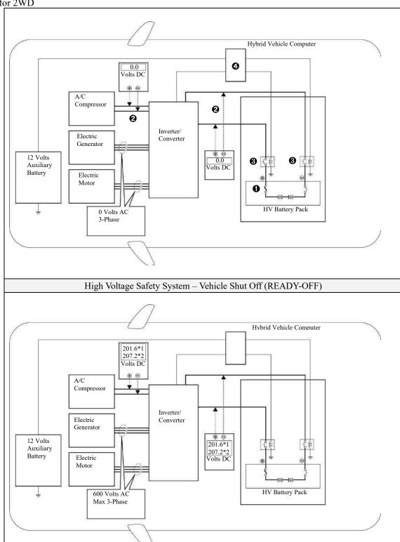
High Voltage Safety System - Vehicle On and Operational (READY-ON)
