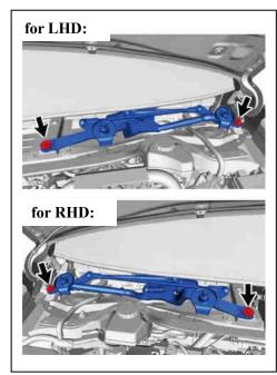
(2) Disengage the motor grommet as shown in the illustration.
