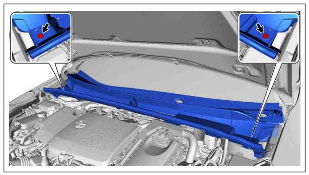
(2) Disengage the guide as shown in the illustration.
