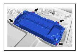
Hold the areas shown in the illustration and lift the HV battery.
