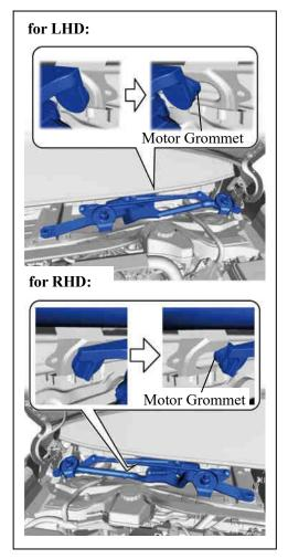
(3) Disconnect the connector to remove the windshield wiper motor and link assembly.
