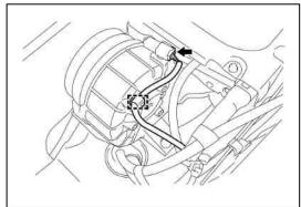
(2) Remove the 2 bolts, nut and battery cooling blower assembly.
