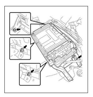
(3) Remove the HV battery.
