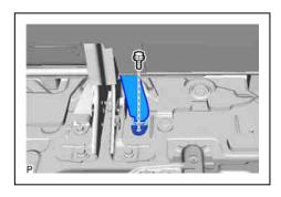
(4) Remove the seat inner belt sub-assembly from the rubber band of the rear seat cushion assembly as shown in the illustration.
