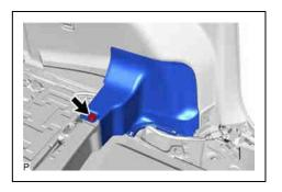
(2) Disengage the 5 clips and 3 guides to remove the front deck side trim cover LH as shown in the illustration.
