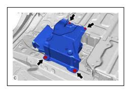
(3) Disengage the 2 claws to remove the blower sub-assembly from the HV battery.
