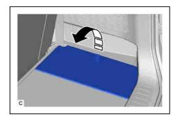
(2) Disengage the 6 claws and 2 guides to remove the battery service hole cover.
