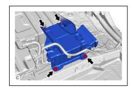
(4) Disengage the 2 claws to remove the blower sub-assembly from the HV battery.
