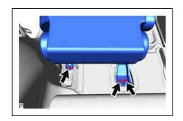
f) Disengage the 2 pins and remove the rear No. 1 seat assembly LH.
