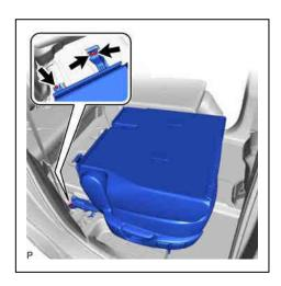
f) Disengage the 2 pins and remove the rear No. 1 seat assembly RH.
