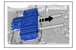
(10) Pull out the HV battery to the rear of the vehicle at the positions shown in the illustration.
