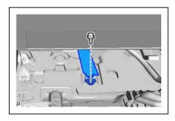
(4) Remove the rear No. 2 seat inner belt sub-assembly RH from the rubber band of the rear seat cushion assembly as shown in the illustration.
