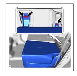
f) Disengage the 2 pins and remove the rear No. 1 seat assembly LH.
