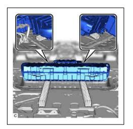
(5) Remove the clip and No. 2 HV battery intake duct LH from the HV battery.
