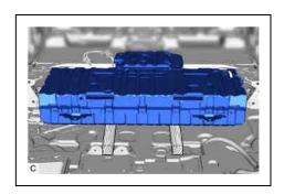
(11) Using a suitable adaptor such as straps, remove the HV battery while tilting it.
