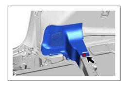
(2) Disengage the 5 clips and 2 guides to remove the front deck side trim cover LH as shown in the illustration.
