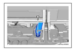
(4) Remove the rear No. 2 seat inner belt sub-assembly LH from the rubber band of the rear seat cushion assembly as shown in the illustration.
