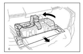
(10) Using a suitable adaptor such as a rope, remove the HV battery while tilting the HV battery.
