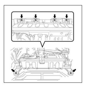
(2) Pull the HV battery toward the center of the luggage compartment.
