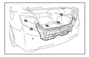
(2) Disengage the 4 clips and remove the rear floor finish plate.
