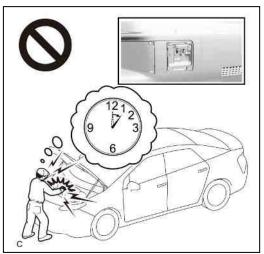
• Place a "HIGH VOLTAGE WORK IN PROGRESS. DO NOT TOUCH. " sign, in order to prevent other technicians from accidentally reconnecting the power while work is in progress.
