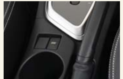
Pushing the Sport button in CVT models alters engine and transmission characteristics for a sportier response.
