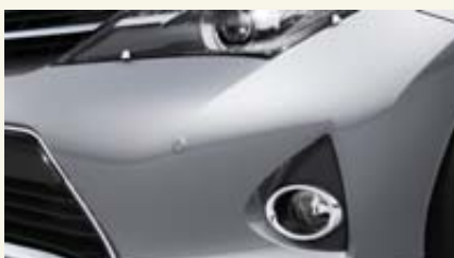
Front Park Assist. This four sensor Front Park Assist system provides audible alerts to help assist with front clearance when parking. The ultrasonic sensors are colour matched to the vehicle.
